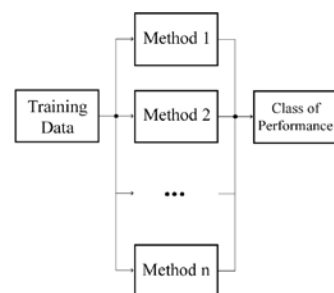
FIGURE. 3 PARALLEL ARCHITECTURE FOR COMBINING CLASSIFIERS.
