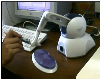
FIGURE. 1 A HAPTIC DEVICE USED IN VR SYSTEMS.
